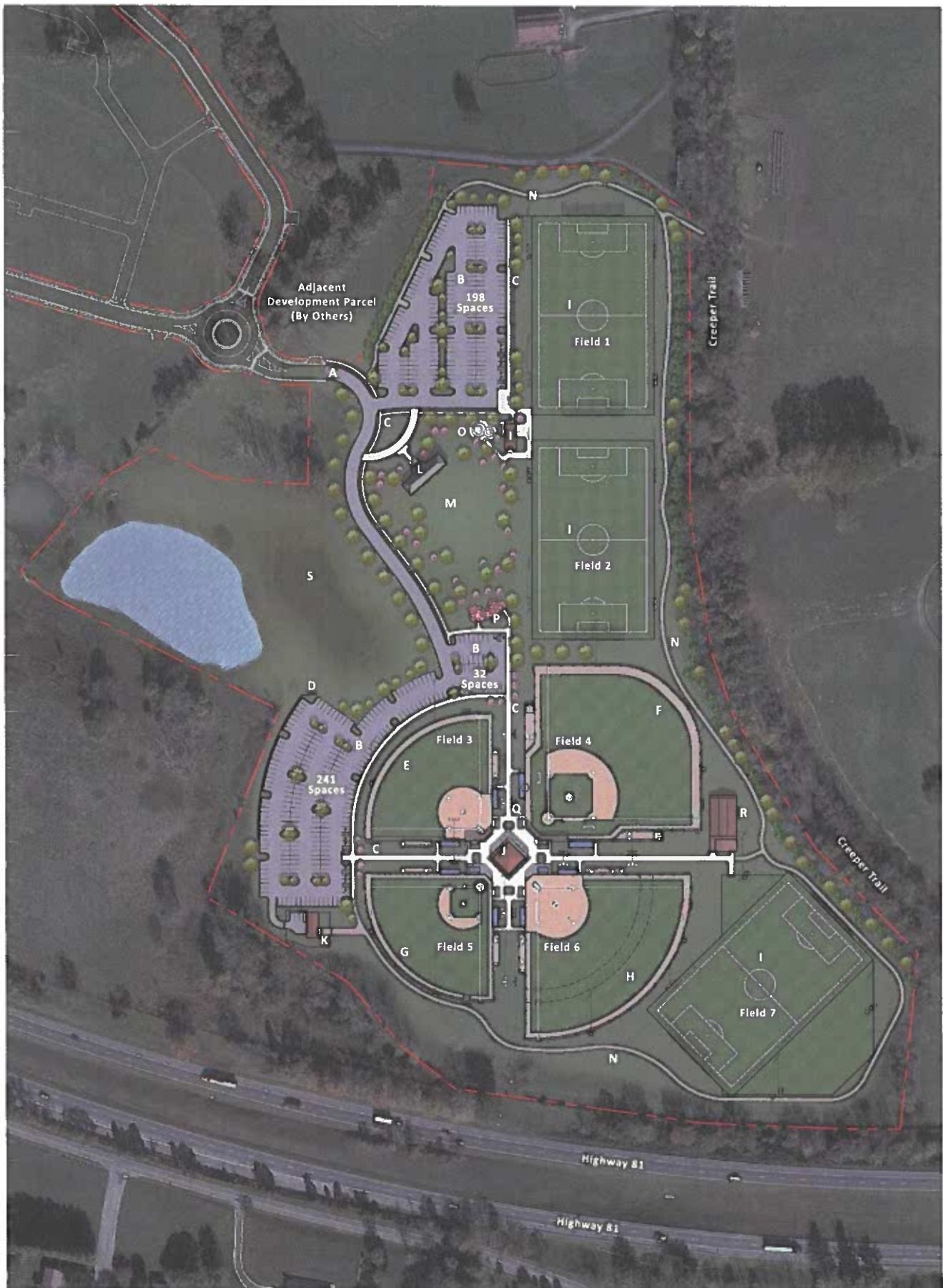
A. Entry Drive B. Parking Lot C. Sidewalks D. Retaining Wall E. 225' Baseball/Softball Field F. 300'/350' Baseball Field G. 225' Baseball Field H. 300' Baseball/Softball Field I. 210'x360' Multi-Purpose Field J. Concession and Restroom Building K. Maintenance Building L. Historic House M. Open Space N. Walking Trail O. Splash Pad P. Playground Q. Bleachers R. Batting Cage Building S. Stormwater
